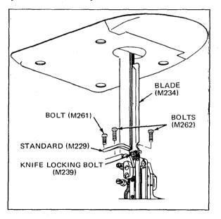
(d) <u>To Replace Inserts</u> - When the Inserts (M253) are worn so badly that there is space to fit two blades between them, they must be replaced.
